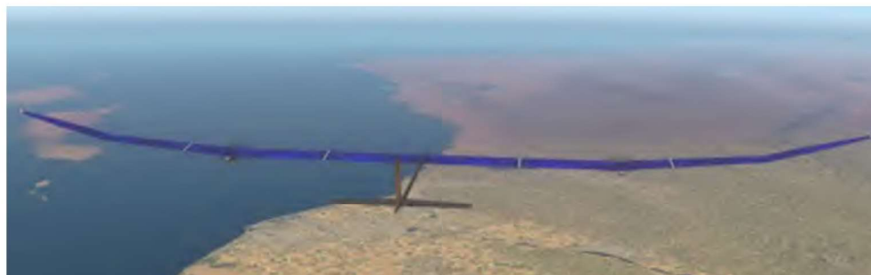
Figure 4 A High Altitude (80k ft), Long Endurance (1 year) UAV with Comms Payload
